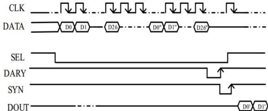
Figure 3 Control Timing Diagram for Amplitude-Phase Multifunctional Chip (Single/Parallel Operation)
